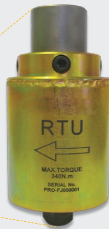
Modification of RTU for Track Bolt Tightening
