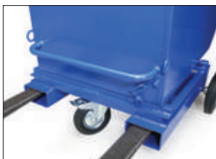
Forklift pockets in two dimensions: Internal dimensions 114 x 54 mm or 150 x 80 mm With full lock (for secure positioning) as standard. For reasons of space, not possible for 250-litre version type B
